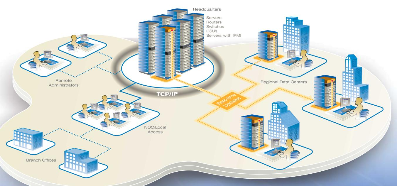
The power of DSView 5 software is its hub and spoke architecture – a fully redundant, replicating database system that includes both SNMP and IPMI proxy appliance support. Users securely authenticate to a central management hub server or one of 15 mirror spoke servers if the primary server is unavailable. This allows for real-time updates and load balancing across multiple sites.
